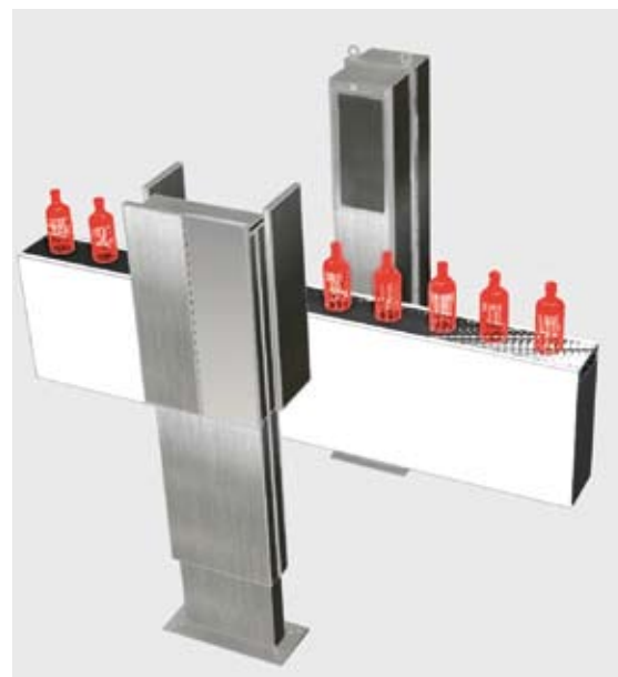
SCHEMATIC SET UP OF THE GVS SYSTEM, CONSISTING OF ONE CAMERA MODULE AND ONE BACK LIGHT MODULE
